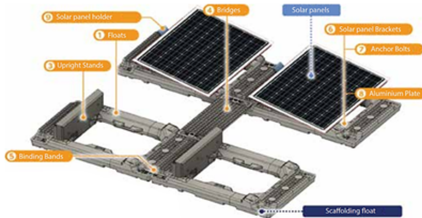
Figure 1.2: Pontoon type floating photovoltaic [1]
